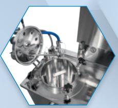
Removable mixing blades with wall's scrapers.
